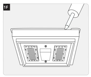
**10** For wet location installation, caulk around the mounting base with waterproof construction sealant.
