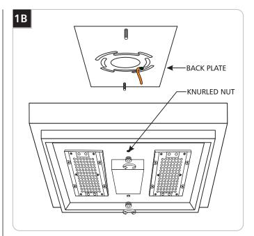
Remove the back plate from the assembly by unscrewing the two knurled nuts.
