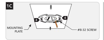
Secure the mounting plate to the electrical box with 2 #8-32 screws.
