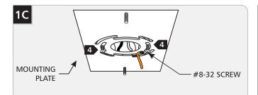
4 Secure the mounting plate to the electrical box with 2 #8-32 screws.
