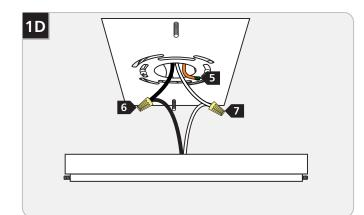
**5** Ground the mounting plate in accordance with local electrical codes.
