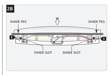
3 Carefully slide the shade pegs into the slots.
