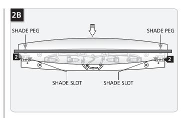
2 Carefully slide the shade pegs into the slots.
