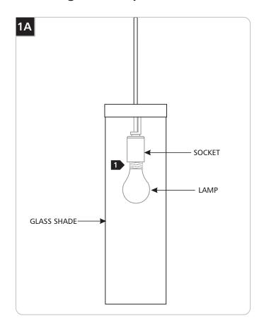
**CAUTION:** To reduce the risk of a burn or electric shock during relamping, disconnect the power to the fixture.
