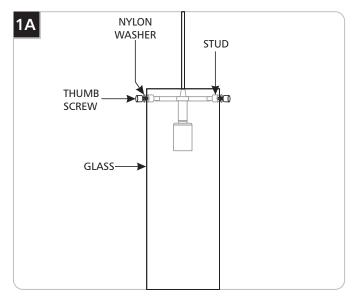
1 Line up the holes in the glass with the arms on the socket base.
