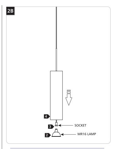
Use **MAX** 50 Watt, MR16 Front Cover Halogen Lamp.
