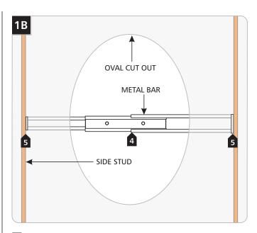
4 Center the metal bar vertically in the oval cut out.
