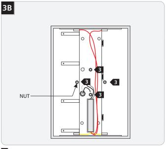
Mount the pan to the backplate with the provided washers, lock washers and nuts.
