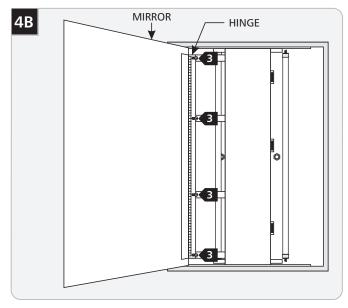
Carefully attach the mirror hinge onto the fixture and tighten all four screws.
