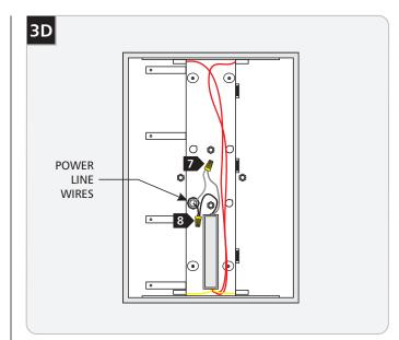
Connect the neutral power line wire to the white fixture wire with a wire nut.
