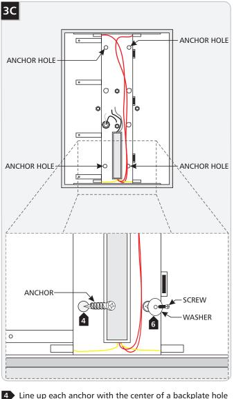
Line up each anchor with the center of a backplate hole and push the anchor in up to the threads.
