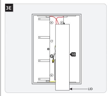
10 Replace the lid onto the center housing and tighten the screws.
