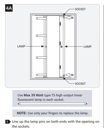
2 Insert the pins all the way into the sockets and rotate the lamp to lock it in place.
