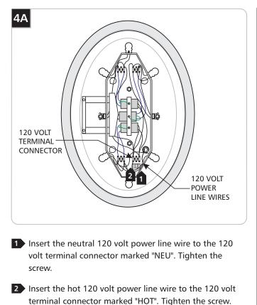
In accordance with local electrical codes connect the ground.
