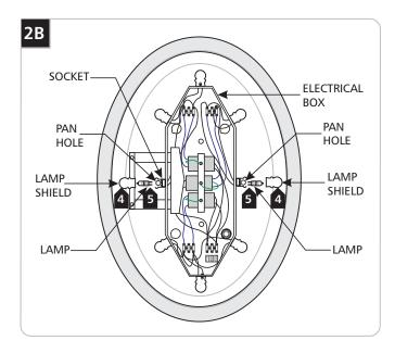
4 On the left and right side of the electrical box pull out the lamp shields.
