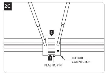
2 Slide the fixture connectors toward each other so that the plastic pins on the fixture connector slips into the side hole on the opposite fixture connector.
