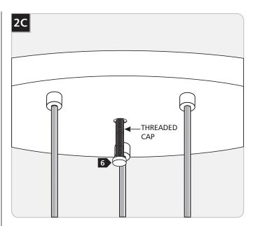
6 Secure the fixture canopy to the electrical box with the threaded cap.
