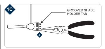
4 If the Prism glass shield fits tight onto the fixture, then carefully bend the grooved shade holder tabs in slightly with the needlenose pliers. If it fits loose, then carefully bend the grooved shade holder tabs out slightly with the needlenose pliers.
