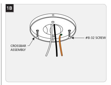
2 Mount the crossbar to the electrical box with the two #8-32 screws provided.
