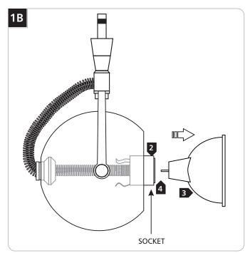
Use **MAX** 50 Watt, MR16 Front Cover Halogen Lamp.
