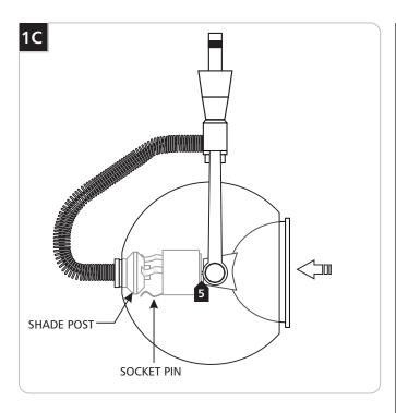
5 Snap the socket pins onto the shade post by pushing the lamp into the shade.
