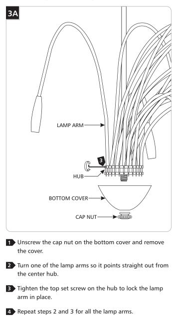
5 Install the bottom cover and screw the cap nut back on.
