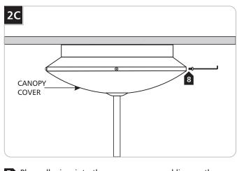
Place all wires into the canopy cover and line up the canopy cover holes with the backplate holes.
