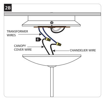
Connect the canopy cover wire to one 12 volt transformer wire and the chandelier wire to the other 12 volt transformer wire with wire nuts.
