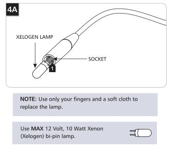
**1** Push the lamp pins all the way into the socket.
