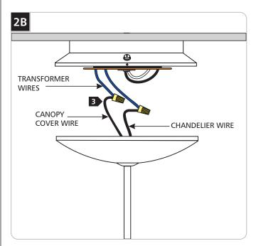
Connect the canopy cover wire to one 12 volt transformer wire and the chandelier wire to the other 12 volt transformer wire with wire nuts.
