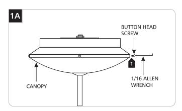
Remove the four button head screws around the chandelier canopy with provided 1/16 Allen wrench.
