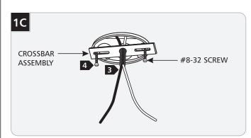
**3** Feed the 120 volt power line wires through the nipple attached to the crossbar.
