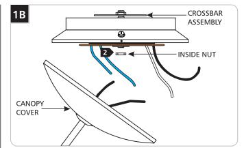
2 Unscrew the inside nut to remove the crossbar assembly. Do not disassemble the nipple from the crossbar.
