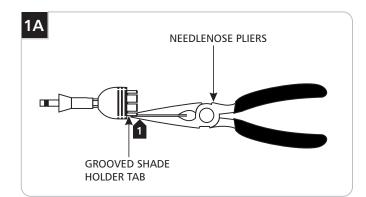
If the accessory shade fits tight or loose onto the Tilt fixture, then carefully bend the grooved shade holder tabs in or out slightly with needlenose pliers.
