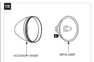
2 Insert the MR16 lamp into the proper accessory shade.
