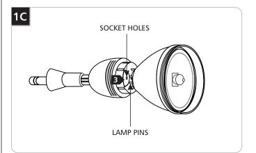
Line up the lamp pins with the socket holes. Insert the MR16 lamp pins into the socket holes, simultaneously push the accessory shade onto the grooved shade holder.
