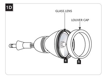
Place the optional louver or glass lens accessory into the louver cap (This applies only for Round Glass Back Shield or Cone Glass Shield).
