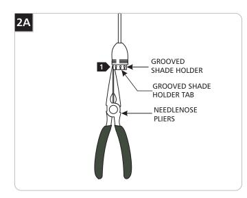
1 If the accessory shade fits tight or loose onto the Torpedo pendant, then carefully bend the grooved shade holder tabs in or out slightly with needlenose pliers.
