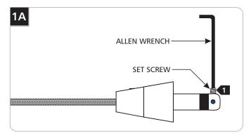
Back out (do not remove) the set screw on tip of the connector with the provided Allen wrench.
