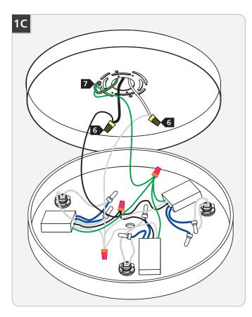
6 Connect the black wire to the hot power line wire and the white wire to the neutral power line wire with wire nuts.
