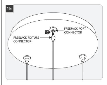
Screw the FreeJack fixture connector completely into the FreeJack port connector.
