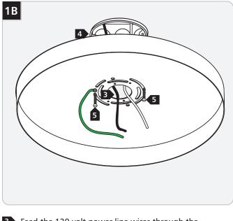
Feed the 120 volt power line wires through the mounting plate center hole.
