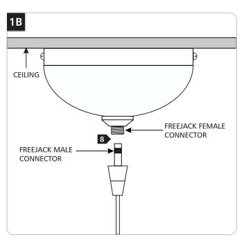
8 Screw the fixture FreeJack male connector into the FreeJack female connector.
