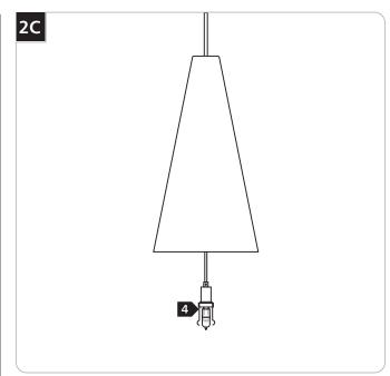
Use MAX 50 Watt, Bi-Pin Halogen Lamp.
