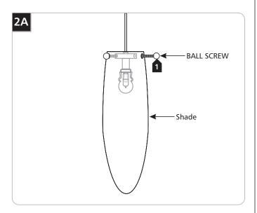
1 To remove the shade, hold the shade with one hand and unscrew the three ball screws with the other hand.
