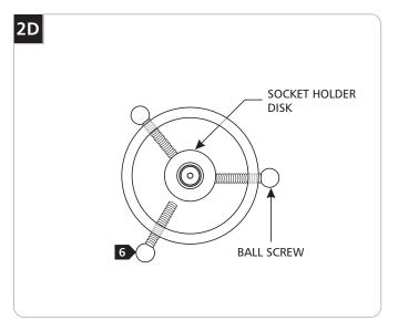
With one hand hold the shade around the socket holder disk. With the other hand screw the ball screws into the socket holder disk, do not tighten. Align the socket holder disk in the center of the shade by tightening the ball screws snugly.
