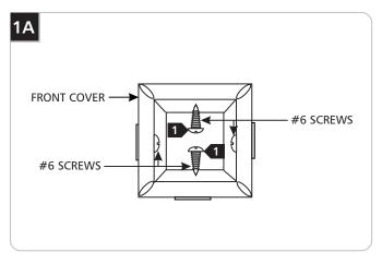
Remove two #6 opposing screws from the front cover of the 2" Electrical box.
