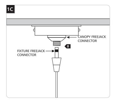
8 Screw the fixture FreeJack connector into the canopy FreeJack connector.
