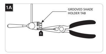
1 If the Belladonna shade fits tight onto the fixture, then carefully bend the grooved shade holder tabs in slightly with the needlenose pliers. If it fits loose, then carefully bend the grooved shade holder tabs out slightly with the needlenose pliers.
