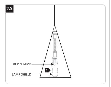
Use MAX 50 Watt, Bi-Pin Halogen Lamp.
