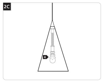
4 Push the lamp shield onto the spring clip.
