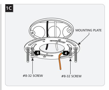
4 Secure the mounting plate to the electrical box with 2 #8-32 screws.
