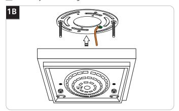
Remove the mounting plate from the fixture base by unscrewing the two knurled nuts.
