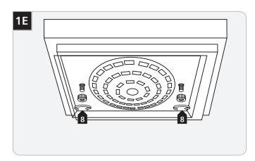
Properly place all wires and wire nut connections into the electrical box, mount the fixture base to the ceiling by reinstalling it onto the mounting plate, and secure it tightly with the knurled nuts.
