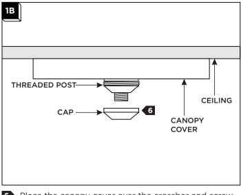
6 Place the canopy cover over the crossbar and screw the cap onto the threaded crossbar post.
