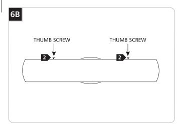
Tighten the two thumb screws on the top of the backplate.
