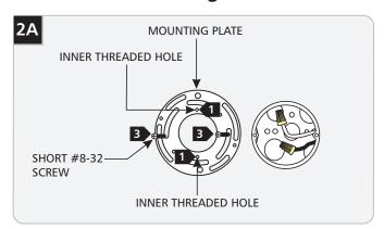
1 Make sure the two inner threaded holes on the mounting plate are positioned vertically.
