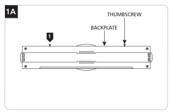
1 Thread in the two thumbscrews into the top of the backplate. Do not fully tighten the thumbscrews.
