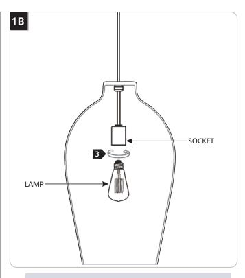
CAUTION: To reduce the risk of a burn or electric shock during re-lamping, disconnect the power to the fixture.
