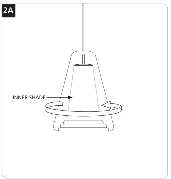
The inner shade may be screwed to lowered or raised it to the desired height.
