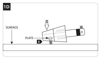
Tap the conical connector on a hard surface with the set screw facing down, so the plate inside drops into place.
