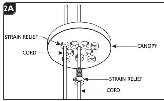
Feed a fixture cord through each the strain relief.
