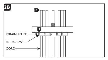
Adjust each fixtures' height (from bottom of the fixture shade to top of the canopy) by pulling the fixture cords through the strain relief.
