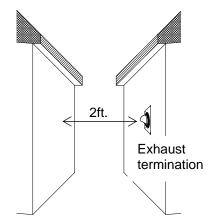
Exhaust and/or direct-vent sidewall terminations should be at least 2 ft. away from an opposite surface/wall. Do not place the termination directly in front of an opening into a building.
