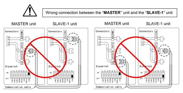
If you connect the "MASTER connector" of the "SLAVE-1" unit to the "SLAVE IN connector" of the "SLAVE-2" unit, the "SLAVE-2" unit will work as an individual unit, and will not be part of the Easy Link system.
