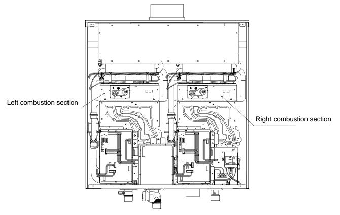
The T-M50 contains two combustion sections. The section that turns on first is whichever section the T-M50 decides is the primary section. The moment at which the secondary section fires will depend on the total flow rate and set temperature of the water heater:
