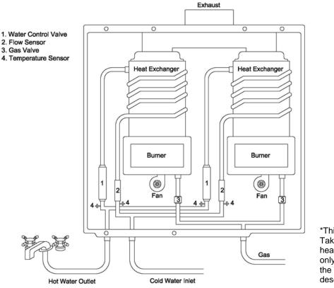
\*This diagram illustrates Takagi's tankless water heater design concepts only and is not accurate to the T-M50's physical description.
