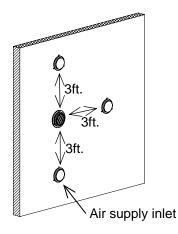
For direct-vent sidewall terminations that use two separate penetrations for the intake and exhaust, distance the intake and exhaust terminations at least 3 ft. away from each other, no matter the orientation.
