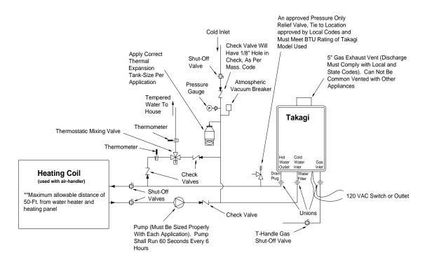
Diagramatic Layout of Radiant Heating and Domestic Water Heater Per Mass. Code
