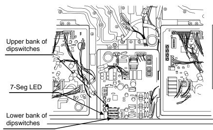
To change dipswitch settings for temperatures, locate the lower bank of dipswitches to the right of 7-Seg LED. DO NOT adjust the upper bank of dipswitches.
