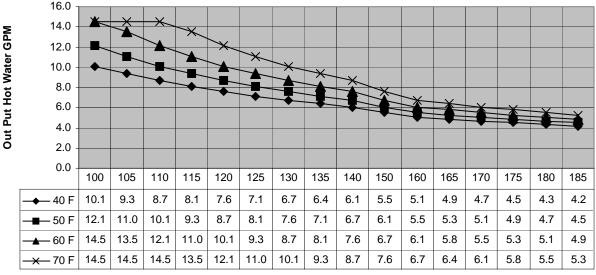
Out Put Temperature vs. GPM (Max. 14.5 GPM) with Various Ground Water Temperature Correct Gas pipe size can be expect this chart
