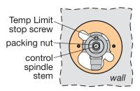
Figure 3 Valve adjustments
