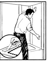
9. Carefully line up front edge of panel with front edge of apron strip (or tub, if strips are not used) with bottom edge resting on the top ledge of the tub. Press firmly starting from bottom and continuing up to insure solid wall contact.
