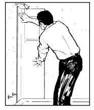
2. For final fit, remove the backing from the pressure sensitive tape and carefully position corner panel. Press firmly to wall...moving hand pressure up and down and side to side, making sure all areas make firm contact to wall. Repeat steps 1 and 2 for installation of the other corner panel.
