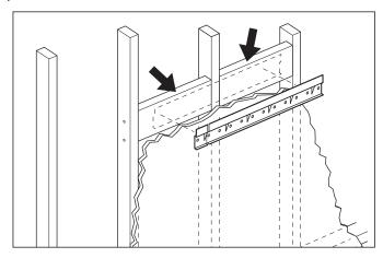
Determine the comfortable working height of the top of the sink. This height may vary depending on your application; however, a typical dimension is 32" up from the floor. Use a level to mark a line 1" below the desired height on the wall.
