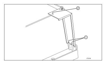
If you have the MF-4W wall mount assembly: Using a flat blade screwdriver, install one panhead screw and washer to hold the filler bracket in place. Do not overtighten the screw.
