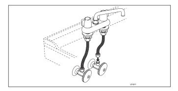
The water lines and waste pipes should now be completely installed.
