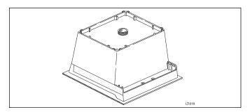
Find the right-side filler bracket. Install it with the end of the filler bracket fitted between the outside of the sink and guide posts (1). Also place the filler bracket over guide post (2) and the screw hole in the bottom of the laundry tub.
