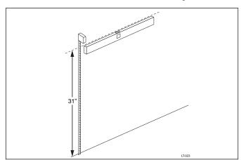
**Note:** Trial fit the wall mounting plate to the laundry tub. If the mounting plate is too long, break off the left side of the wall mounting plate by snapping it along the plate's scored ridge.
