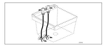
Check all water lines and waste connections for leaks.
