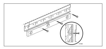
4. Drill a 1/8" pilot hole into the wood and attach the mounting plate to the wall with at least three 1/4" x 1-1/2" long zinc hex head lag screws. Tighten the screws with a Phillips screwdriver.
