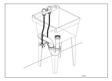
6. Slowly turn ON the hot and cold water shut off valves. Turn the faucets ON and flush the water lines to remove any debris that may be in the water line or the drain pipe.
