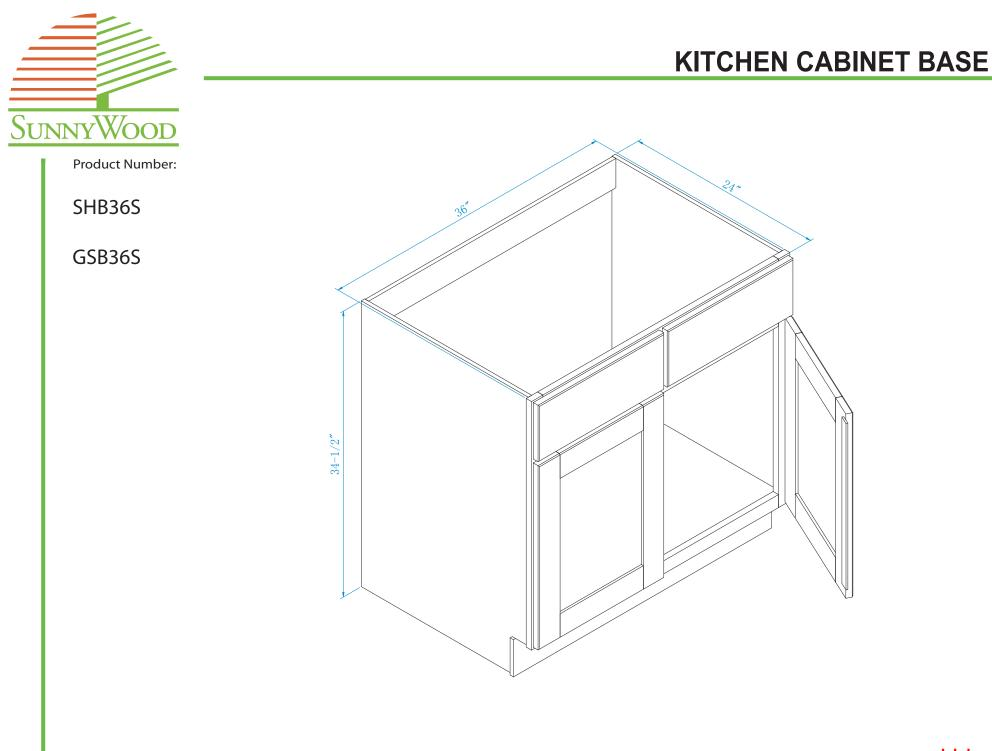
NOTE: No center stile. Batten is attached to door panel in lieu of a center stile.
