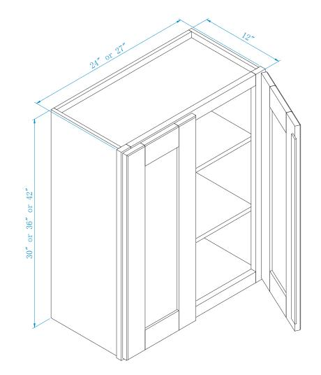
NOTE: No center stile. Batten is attached to door panel in lieu of a center stile.
