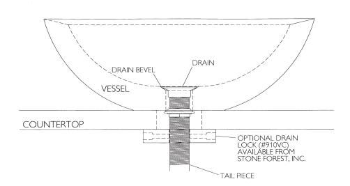
Required drain use 9054D Grid Drain or 9058D Lift and Turn Drain. Drains are 1.25" NPT. This can be supplied by Stone Forest at your request in select finishes.
