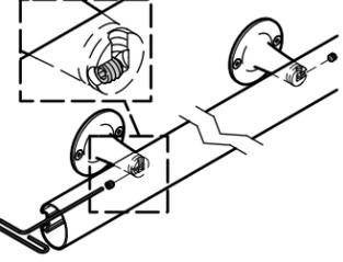
**11** Use silicone sealant to secure the end caps. Remove excess sealant.
