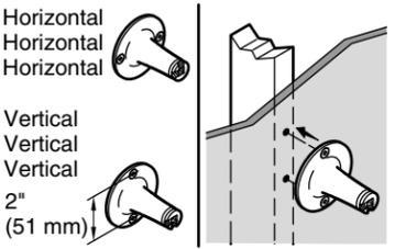
**2** If brackets do not align with studs, install a 1x6 board at the grab bar location.
