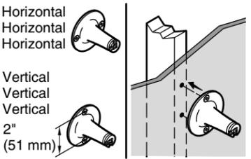
**5 Ceramic Tile:** Drill 1/4" starter holes. Do not drill into the backing!
