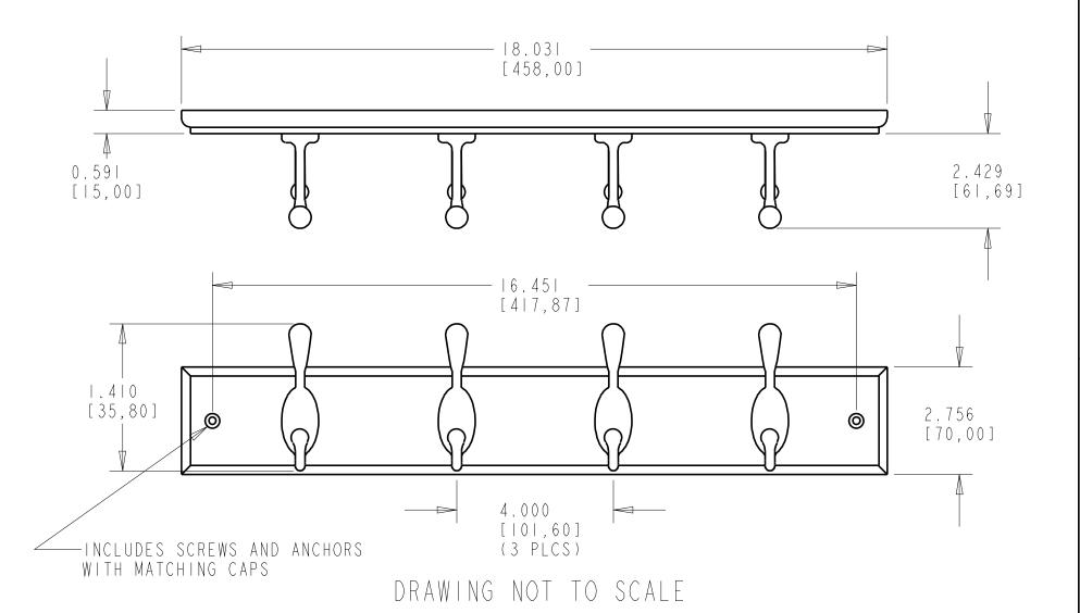
DIMENSIONS IN INCHES AND [mm] SHOWN NOMINAL AND SUBJECT TO CHANGE. FOR CRITICAL SPECIFICATIONS CONTACT STANLEY CUSTOMER SUPPORT. COPYRIGHT STANLEY HARDWARE, 2007
