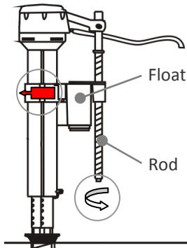
Pull the rod away from the float, as shown. Then, c) adjust the float upwards or downwards, for the desired water level. When complete, d) return the rod into the catch, and twist back 90°; and e) push the red tab back in, to set the float position.
