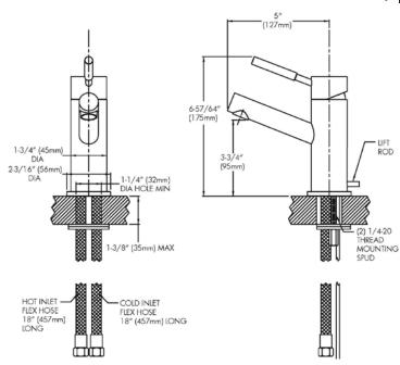
NOTE: 1. All dimensions are in inches (millimeters) unless otherwise specified and are subject to change without notice. 2. Flex hoses have 3/8 compression female threaded connections.
