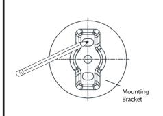
Locate post over Mounting Bracket and tighten Set Screw with Small Flat Tip Screwdriver. Repeat steps 1 thru 5 for remaining items.
