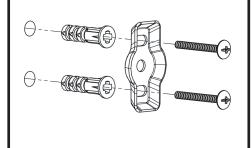
Center Mounting Bracket within traced outline. Mark the 2 mounting locations with a pencil.
