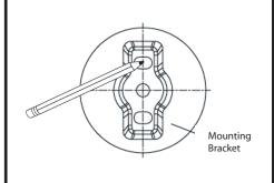
Locate post over Mounting Bracket and tighten Set Screw with Small Flat Tip Screwdriver. Repeat steps 1 thru 5 for remaining items.
