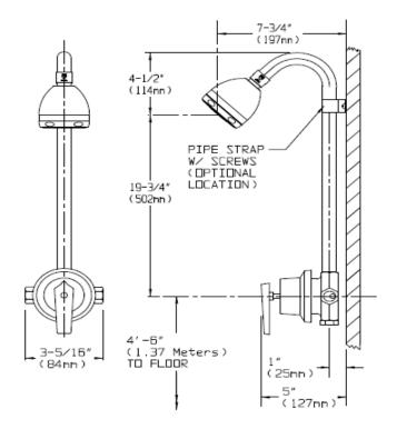
NDTES: 1. ALL DIMENSIONS ARE IN INCHES (MILLIMETERS) UNLESS OTHERWISE SPECIFIED AND ARE SUBJECT TO CHANGE WITHOUT NOTICE, 2. UNLESS OTHERWISE SPECIFIED VALVE INLETS ARE 1/2" NPT FEMALE.
