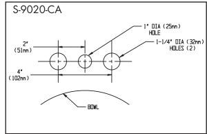
NOTE: 1. All dimensions are in inches (millimeters) unless otherwise specified and are subject to change without notice. 2. Inlet is 3/8" compression with male threads. 3. Position faucet as close to the edge of the sink as possible
