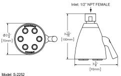
Max. Flow Rate: 2.5 gpm (9.5 L/min)
